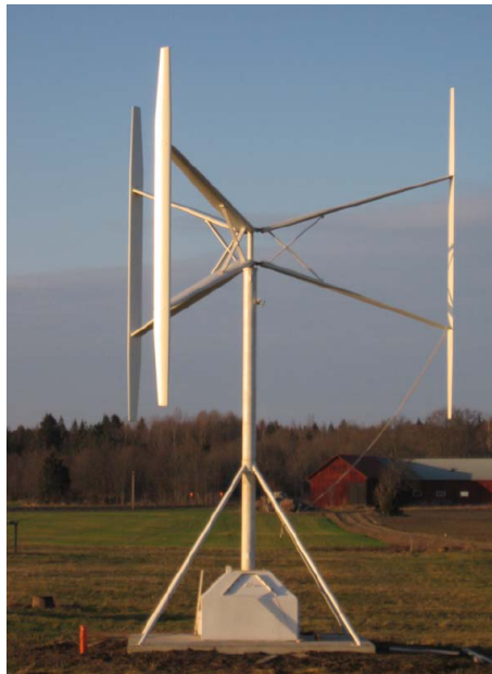
Figure 2.2: The 12 kW H-rotor placed in Marsta.
